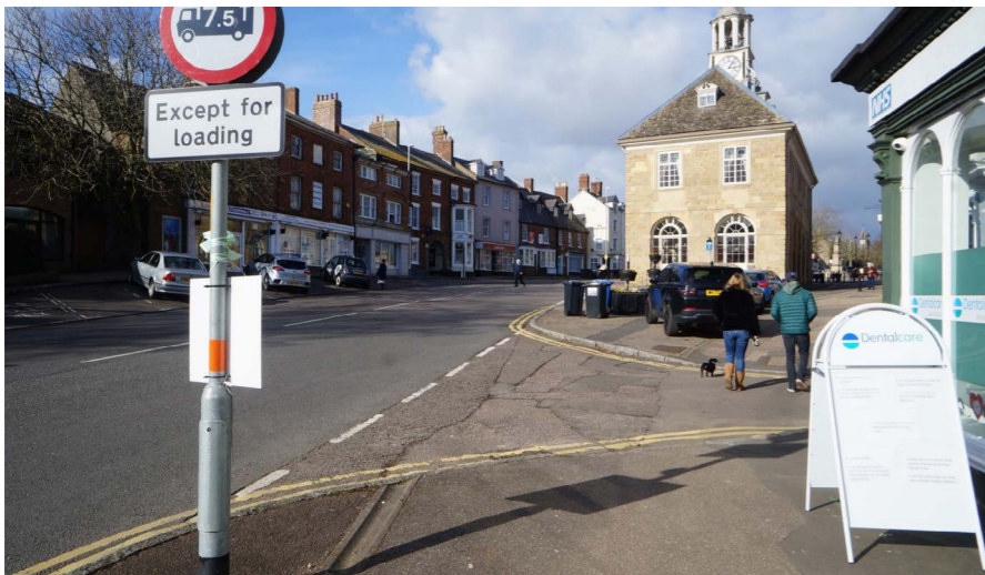
Street clutter, pavement parking and wide junction radii create a poor pedestrian environment on the approach to Market Square
