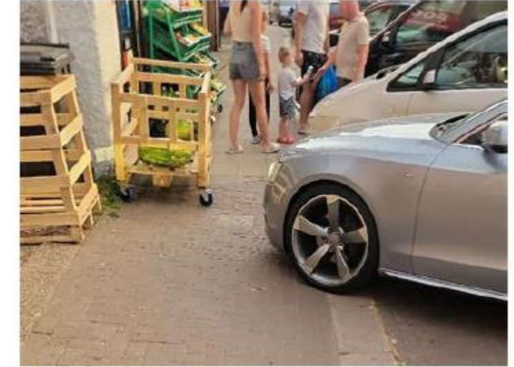
Parked cars encroach onto the footway despite parking bays, made worse by use of the footway as spill out space by the local shop. Echelon parking does not work effectively here
