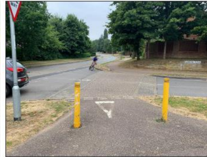
Side road entry treatments help slow turning vehicles and facilitate transitions from the carriageway to shared use facilities.
