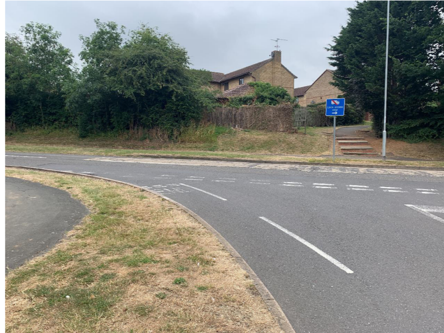
Wide junction radii and inappropriate cycle lanes and the junction of Shackleton Drive and Ashby Road put cyclists in danger of being hooked.
