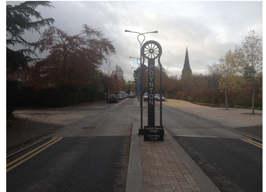
Gateway features, signage and central medians can all contribute to creating a sense of place and reduce traffic speeds to create places where pedestrians and cyclists have more priority
