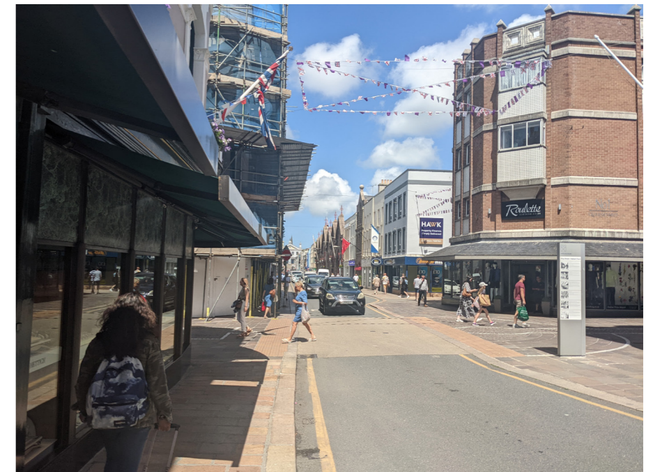
On routes with low traffic speeds and flows, implied or courtesy crossings may be appropriate to provide crossing places between controlled crossings
