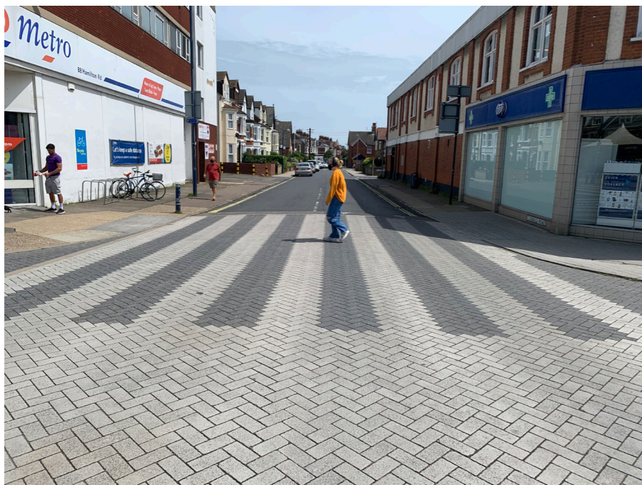
On routes with low traffic speeds and flows, implied or courtesy crossings may be appropriate to provide crossing places between controlled crossings
