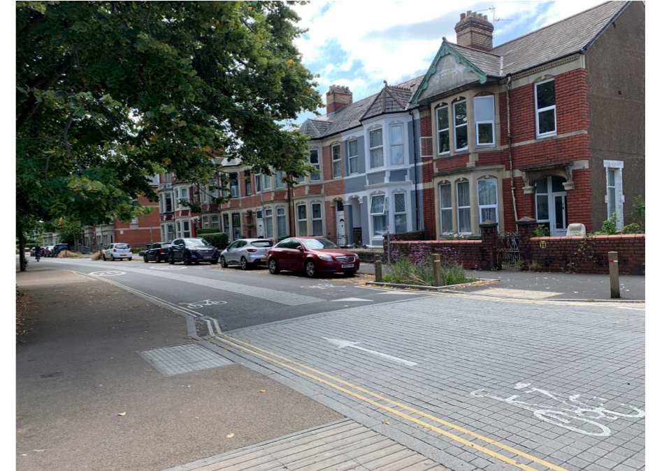
Design cues such as cycle symbols in the carriageway, raised tables and build outs can help slow traffic (Cardiff)
