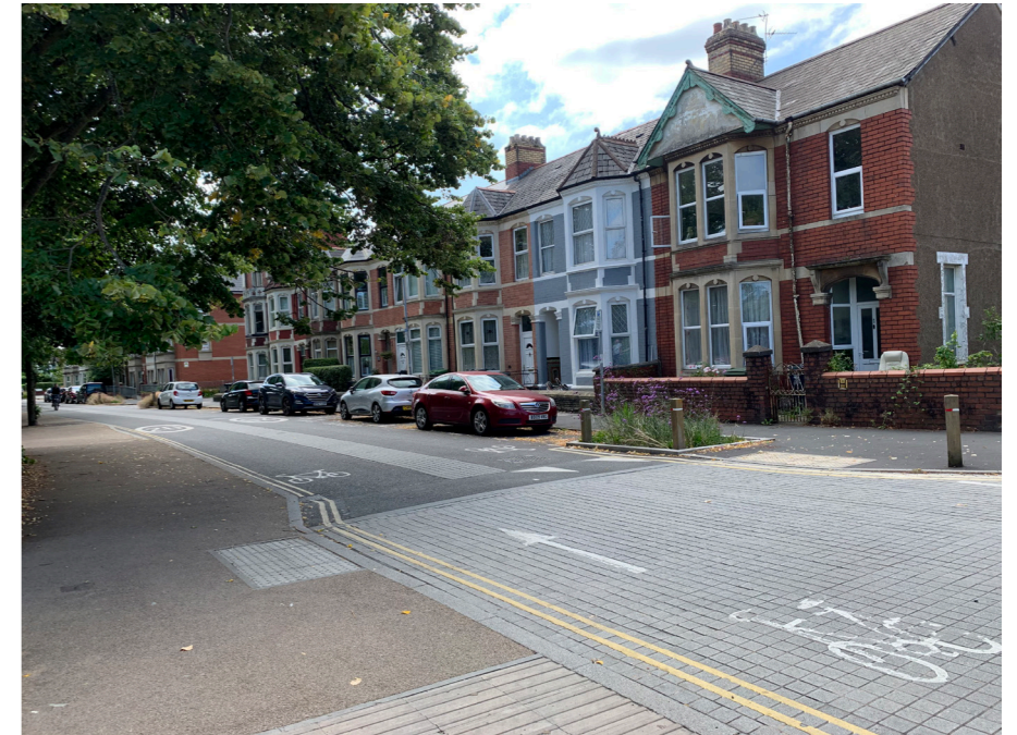
Design cues such as cycle symbols in the carriageway, raised tables and build outs can help slow traffic (Cardiff)
