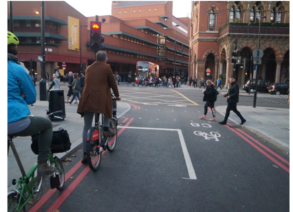
For key cycle routes it might be appropriate to close one or more arms of a junction to general traffic to simplify the junction and provide protected space for cycling
