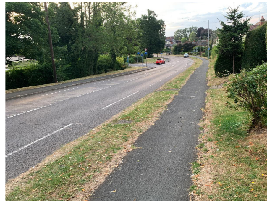
Level differences between the footway and carriageway as well as constrained sections mean that it is not possible to provide protected cycling infrastructure along the route.
