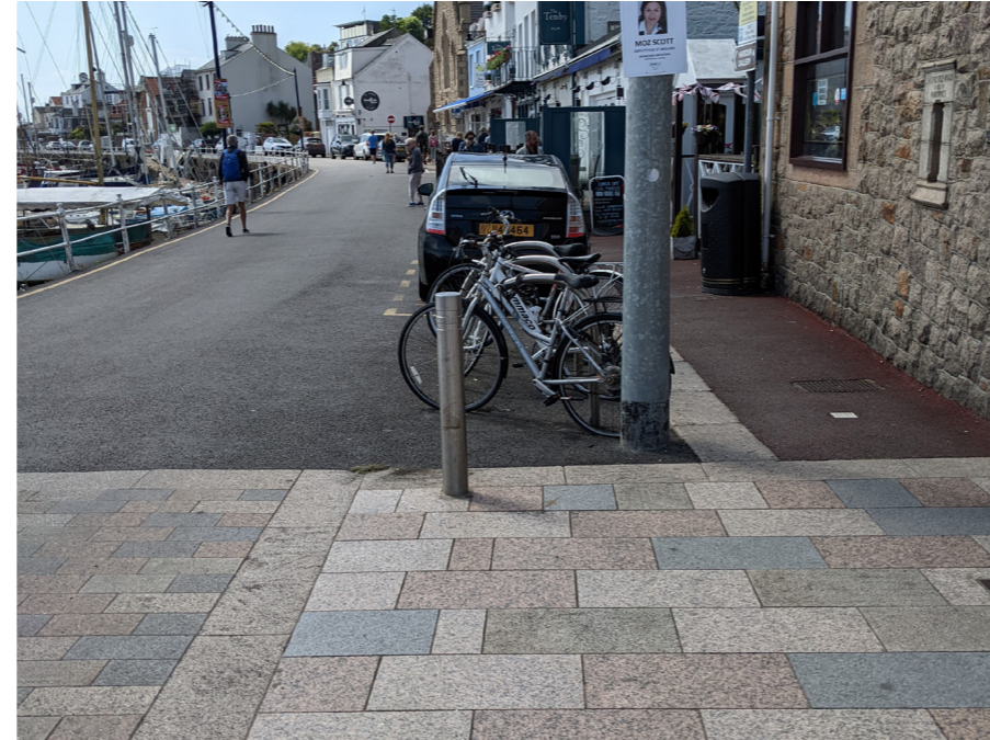
In town centres, cycle parking should be provided at regular intervals. Where possible, cycle parking should be placed in the carriageway rather than footways
