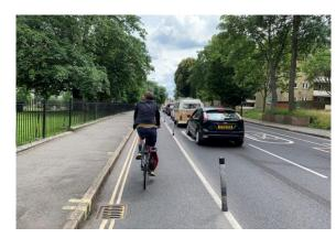
Light segregation using flexible bollards is a cost-effective way of created protected space for cycling (Green Lanes)
