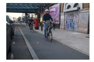
With-flow cycle track providing kerb-separation
