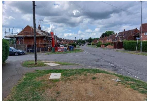
On residential streets like Vernon Road, wide junctions encourage high traffic speeds and cause pedestrians to deviate from their desire line.
