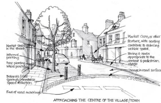
'Traffic in Villages' approach can make sharing the carriageway in small settlements more comfortable and provide placemaking opportunities.
