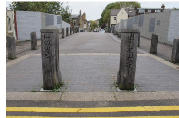
Modal filtering can help reduce traffic significantly ensuring safety for pedestrian and cyclists
