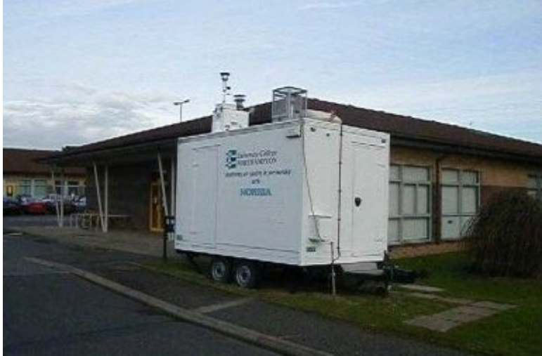
Image of DEFRA Automatic Urban and Rural Network (AURN) national network automatic station at Spring Park, Northampton
